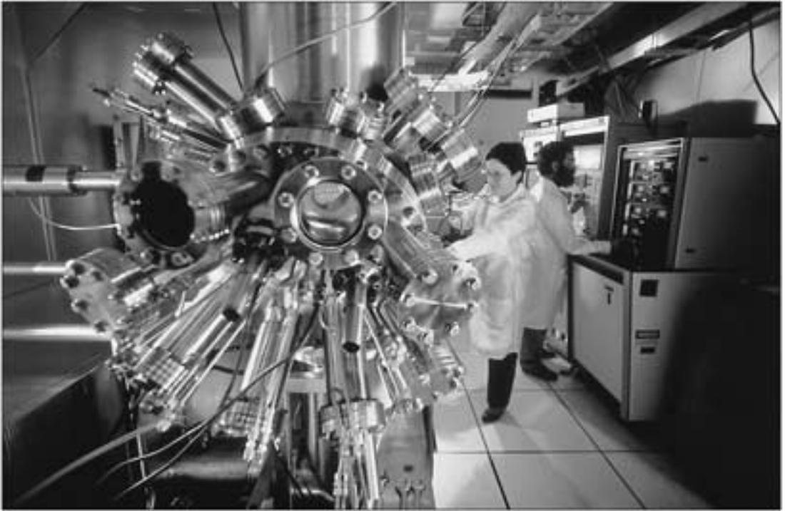
A Molecular Beam Epitaxy (MBE) unit used to make integrated microchips. AT&T Bell Labs/SPL/Cosmos
